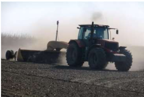
Figure 8 – Special tools and machines used for rice fields leveling: lazer (a), leveling complex "Mara" (b)
